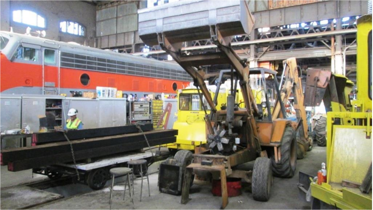
The back-hoe sans radiator and engine shroud
