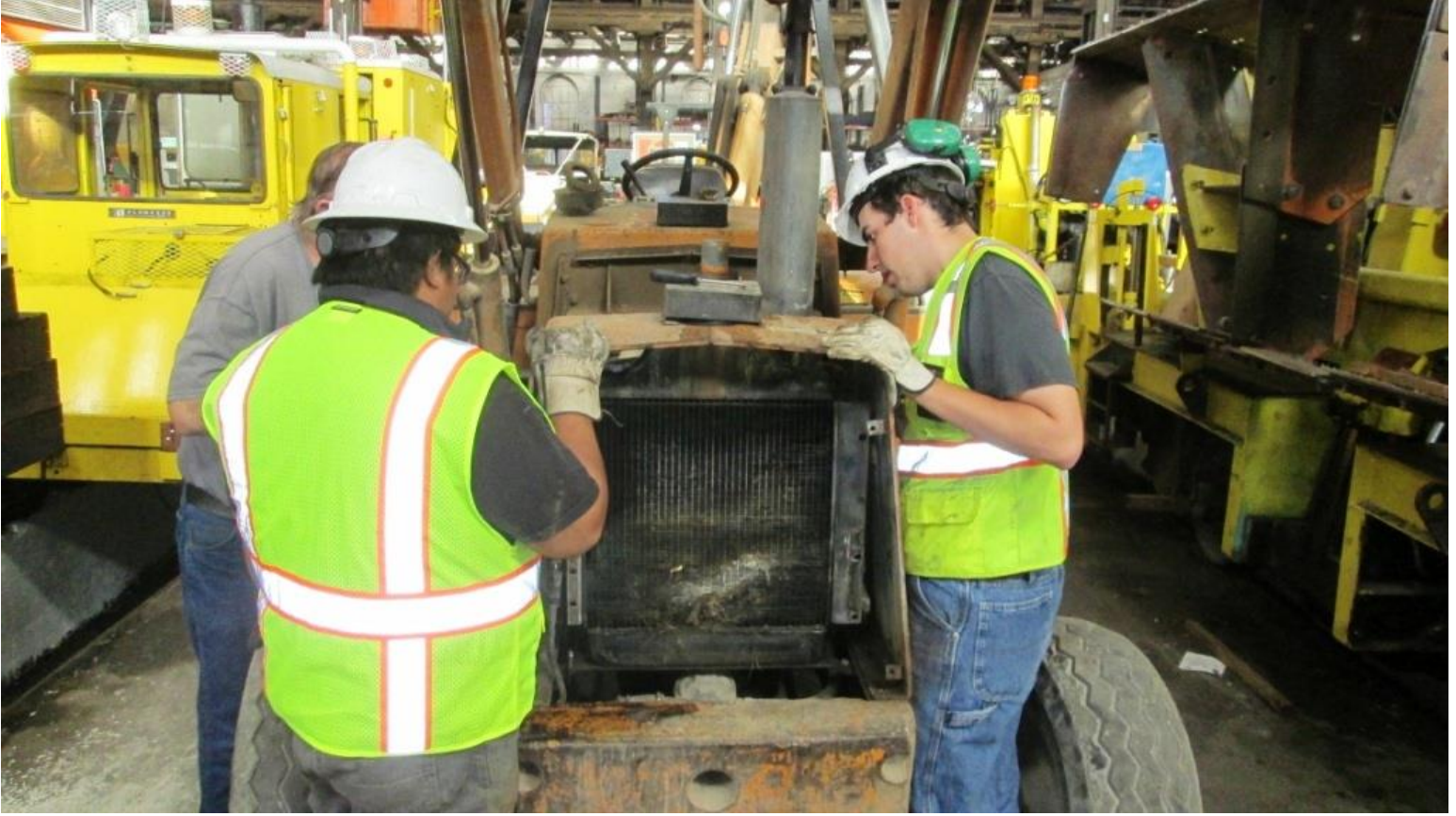
Anthony and Weston remove the front end of the back-hoe
